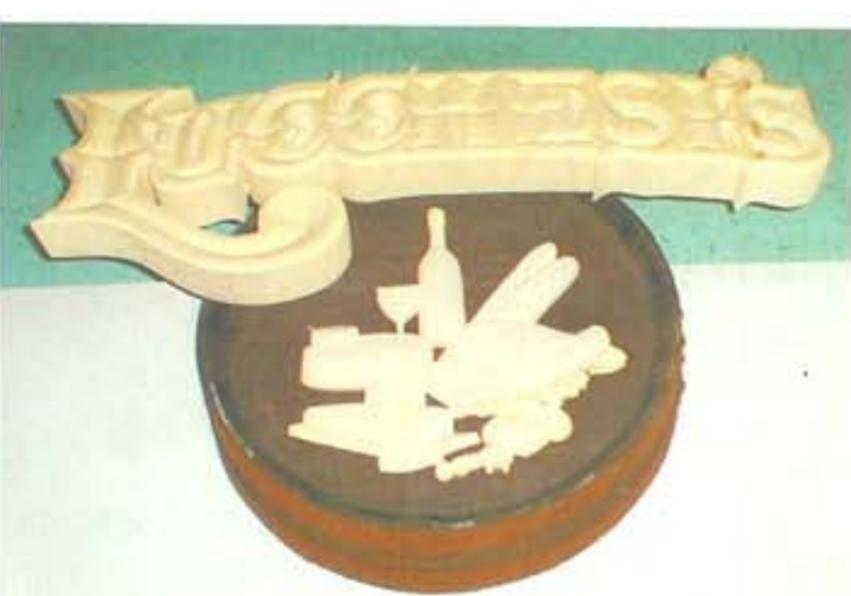
Ron adhered the text and pictorials, made of 15-lb. HDU, to a 12-in.-deep barrel using an aluminum, split-L bracket.
