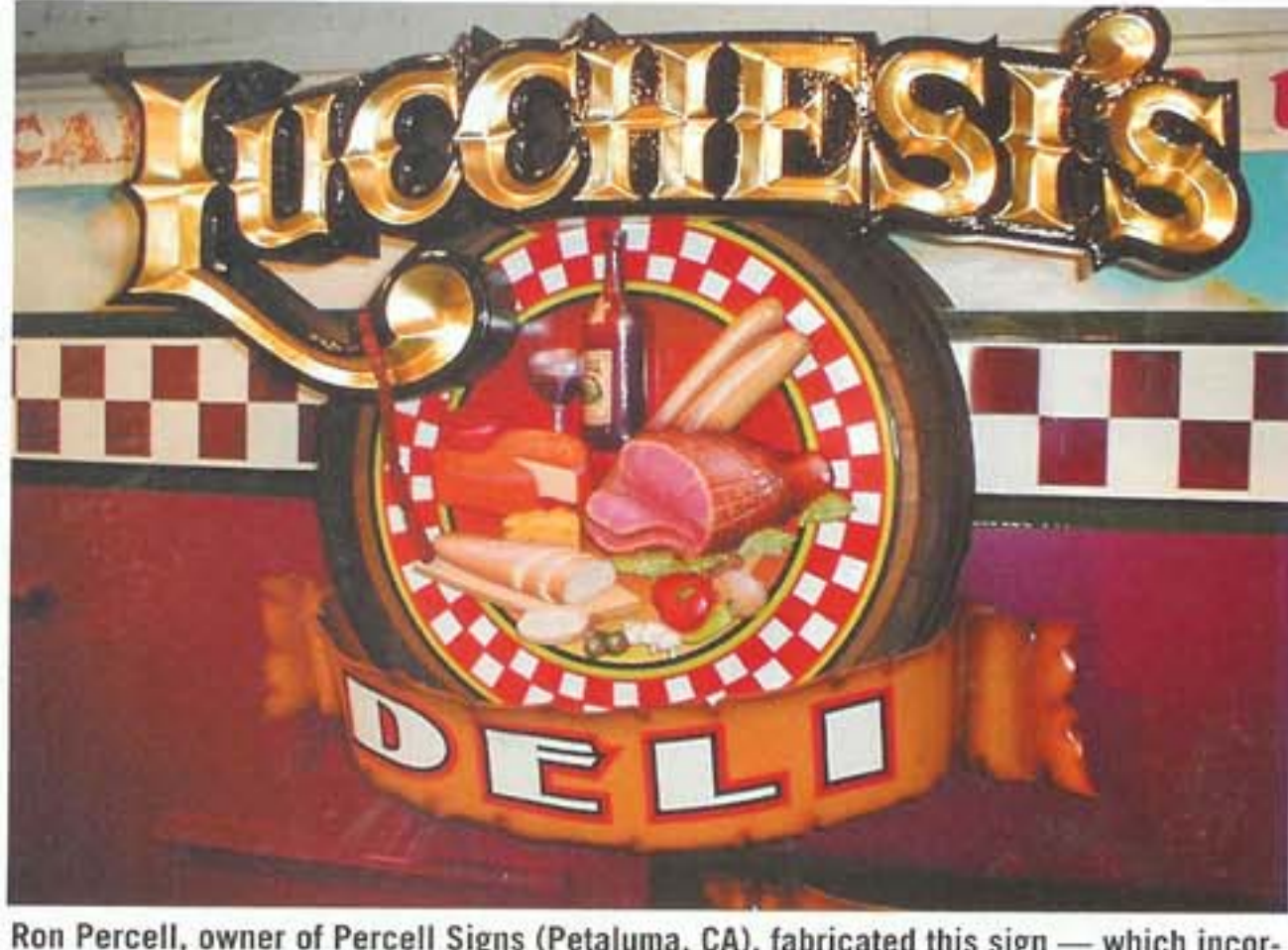
Ron Percell, owner of Percell Signs (Petaluma, CA), fabricated this sign — which incorporates PVC, Sign*Foam® high-density urethane (HDU), Styrofoam® polystyrene foam, digitally imaged vinyl and magnetic materials, and a mixture of lettering enamel and clearcoat — for a local deli moving into new digs.
